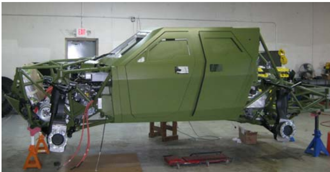
Figure 4 - FED BRAVO Tubular Space Frame and Cab
